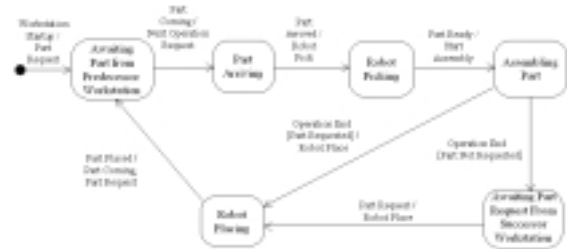
Example of Statechart for High Volume Workstation Controller
